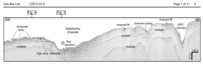
Fig. 5 Deep towed sub-bottom profiler image adjacent to east wall of GPC. Noted that sub seafloor high reflective amplitude strata are accompanied by series of erosional gullies and channels in the Xiaoliuchiu channel
